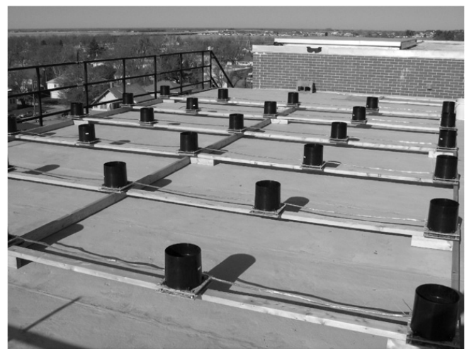
Fig. 1. A photograph of part of the rain gauge array used to acquire data in this experiment. Each of the black canisters is calibrated and leveled tipping-bucket rain gauges. Accumulations for each gauge were recorded and analyzed using a customized data-recording system run from a computer in the adjacent penthouse.
