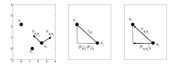
The left figure shows the position of the three charges, and I've already figured out the directions of the two forces acting on  $q_3$ , noting that the force between  $q_1$  and  $q_3$  must be
