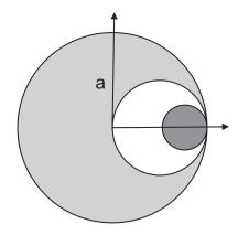
8. A thin uniform circular lamina with diameter D has a smaller circle cut out from it – this time with diameter d. The smaller circle is tangent to the larger circle at the outer edge (similar to another problem earlier in this assignment). This system is designed so that the center of mass is exactly at the point directly across from the tangent point of the two circles (See picture below). Find the ratio D/d.
